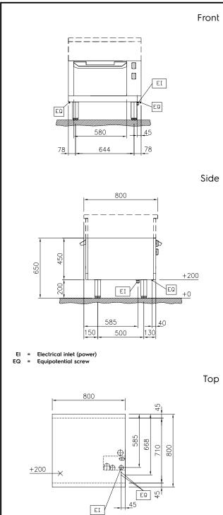
**Electric** Supply voltage: 400 V/3N ph/50/60 Hz Total Watts: 5 kW **Key Information:** Oven working Temperature: 60 °C MIN; 300 °C MAX Oven Cavity Dimensions (width): 575 mm **Oven Cavity Dimensions** (height): 300 mm **Oven Cavity Dimensions** 700 mm (depth): External dimensions, Width: 800 mm External dimensions, Depth: 800 mm External dimensions, Height: 450 mm Net weight: 97 kg Configuration: One-Side Operated Oven GN: GN 2/1
